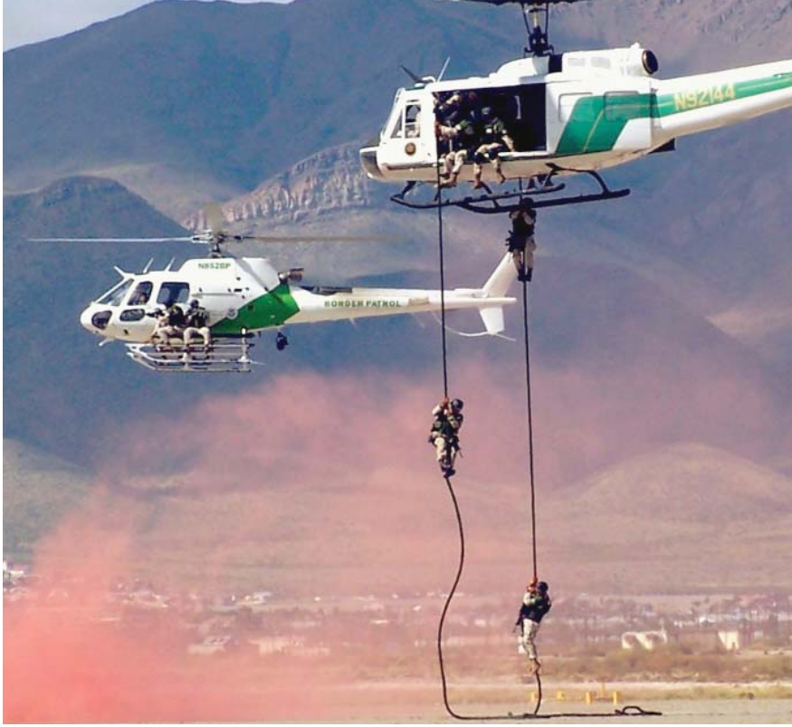
BORTAC marksmen aboard a Eurocopter AS350B3 (L) provide cover from a skid-mounted Tyler Special Ops Platform while operators practice fast roping from the accompanying Bell UH1H.
