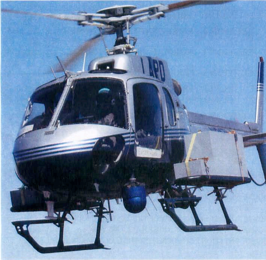
Figure 1 Left Front View of Installed Racks with FLIR & Night Sun
