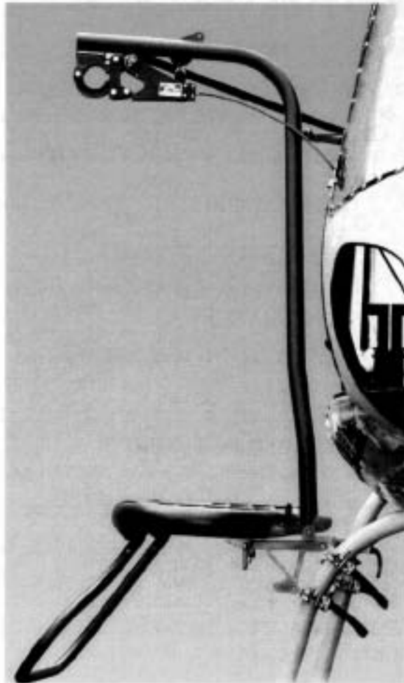
Figure 1 Right Front View of Installed Racks with External Attach Frame
