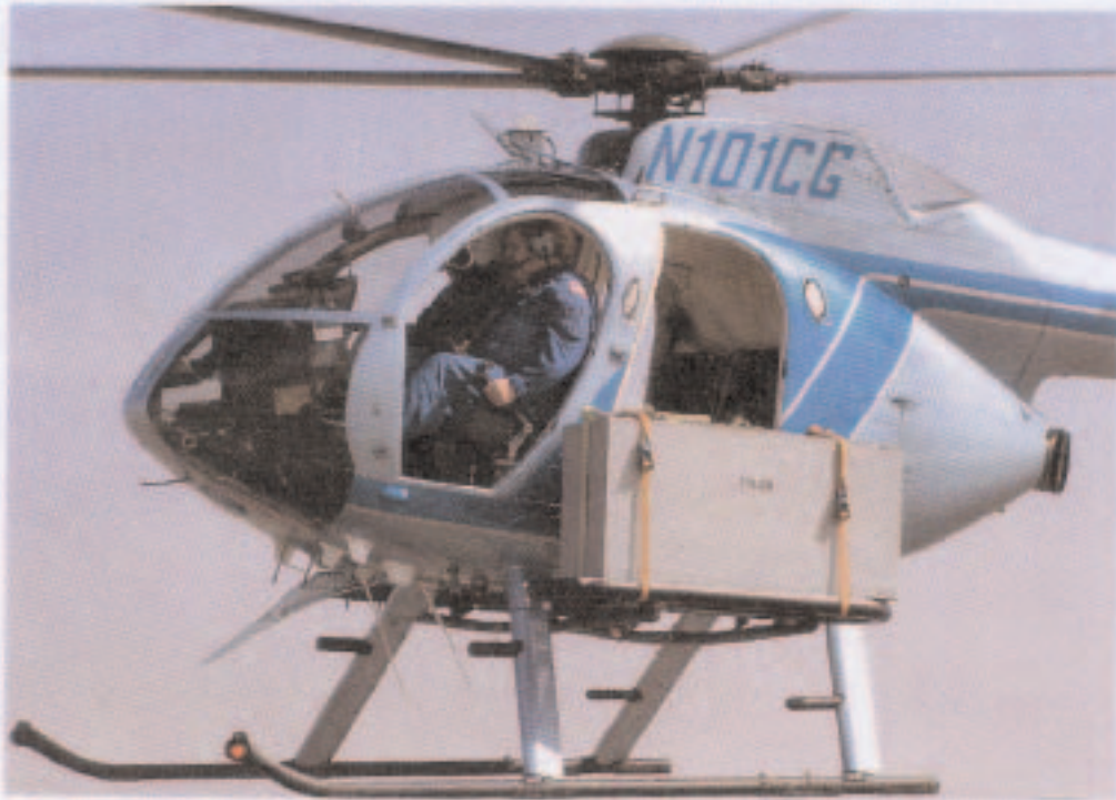
Figure 2 Left Side View of the Installed Racks with Load
