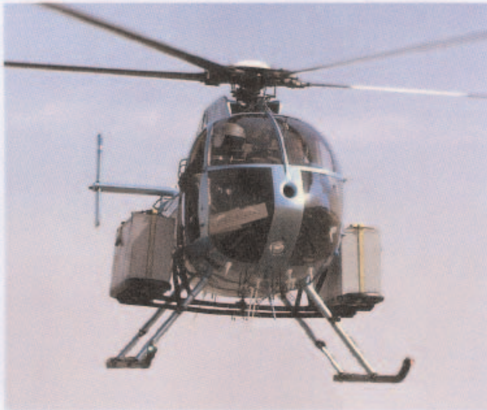
Figure 1 Right Front View of Installed Racks with Load
