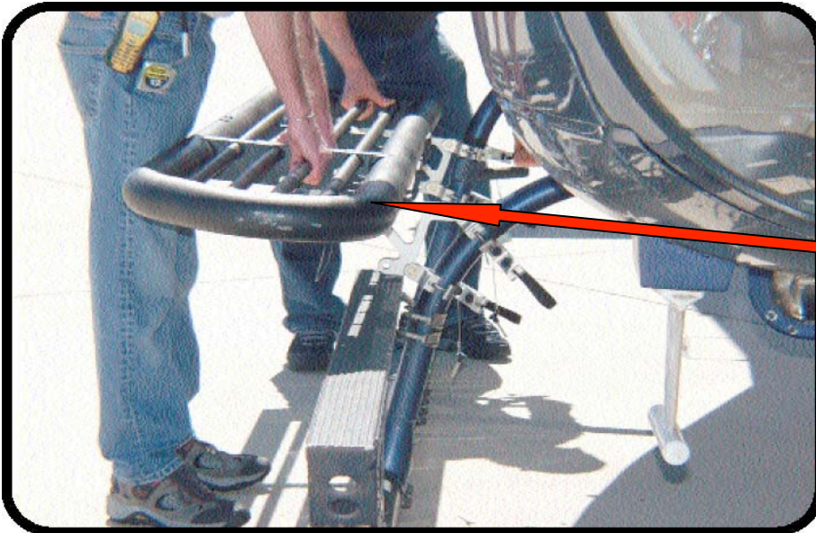
Figure 3.1 Tyler Cargo Rack Installation on the AS350 and 355 series helicopters
