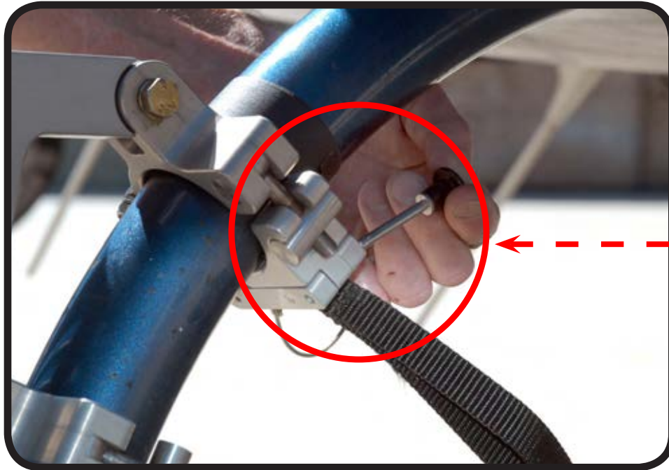
Insert PIP-Pin to secure the clamp lock-arm.
