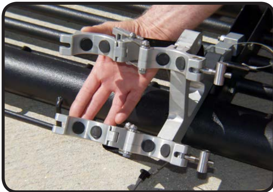
Open skid-gear clamps. (repeat for assembly at other end of cargo rack)
