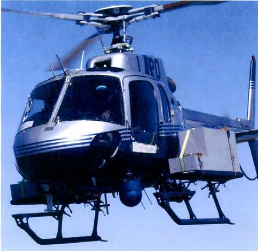
Figure 1 Left Front View of Installed Racks with FLIR & Night Sun
