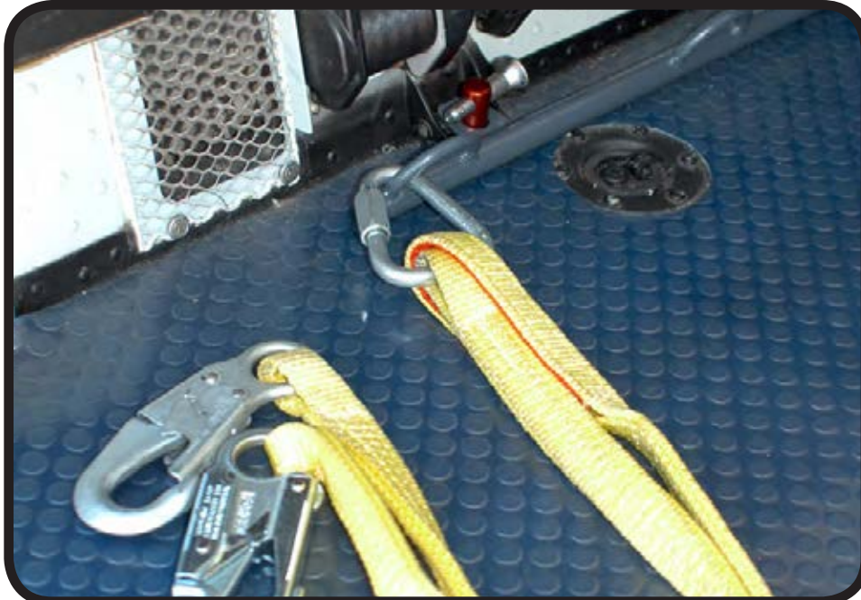
Attach cargo harness-strap to “D-ring” on tie-down bar.
