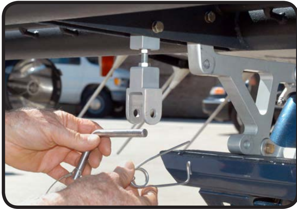
Unlatch and remove safety-clip and lock-rod. (repeat for assembly at other end of cargo rack)
