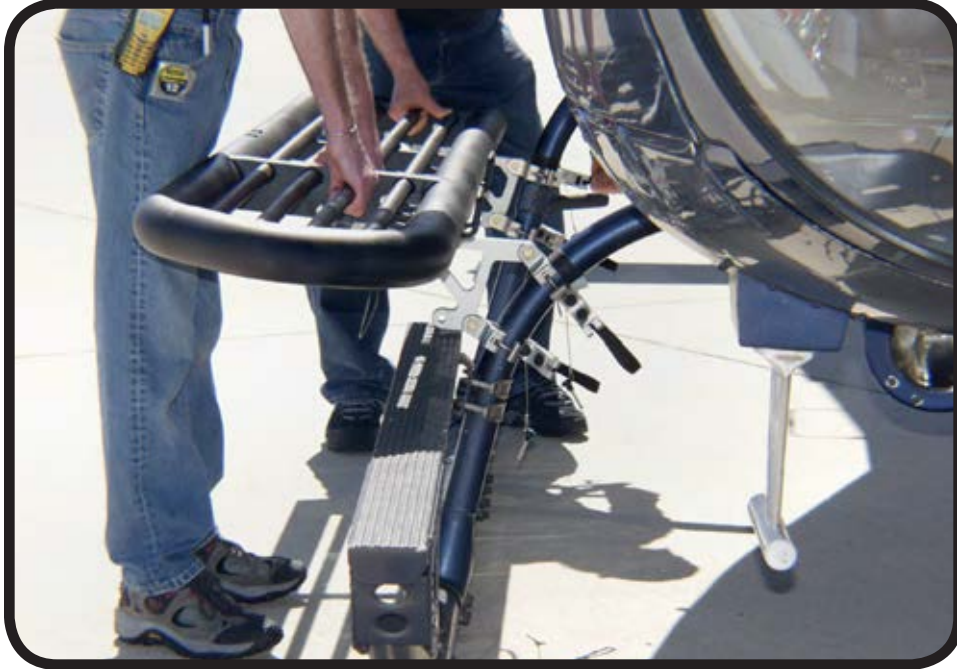
Place skid-gear clamps onto skid support tubes.
