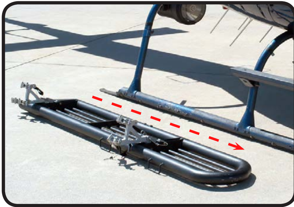
Place Cargo Rack upside-down, near helicopter skid-gear. (Note arrow pointing forward)
