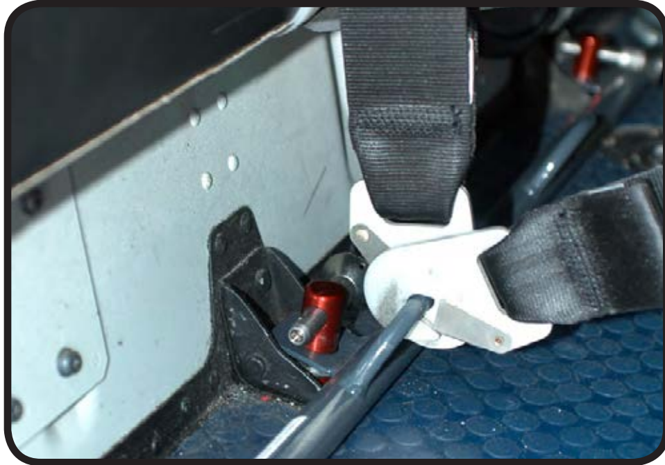
Attach the helicopter seat belts to “D-ring” on tie-down bar.
