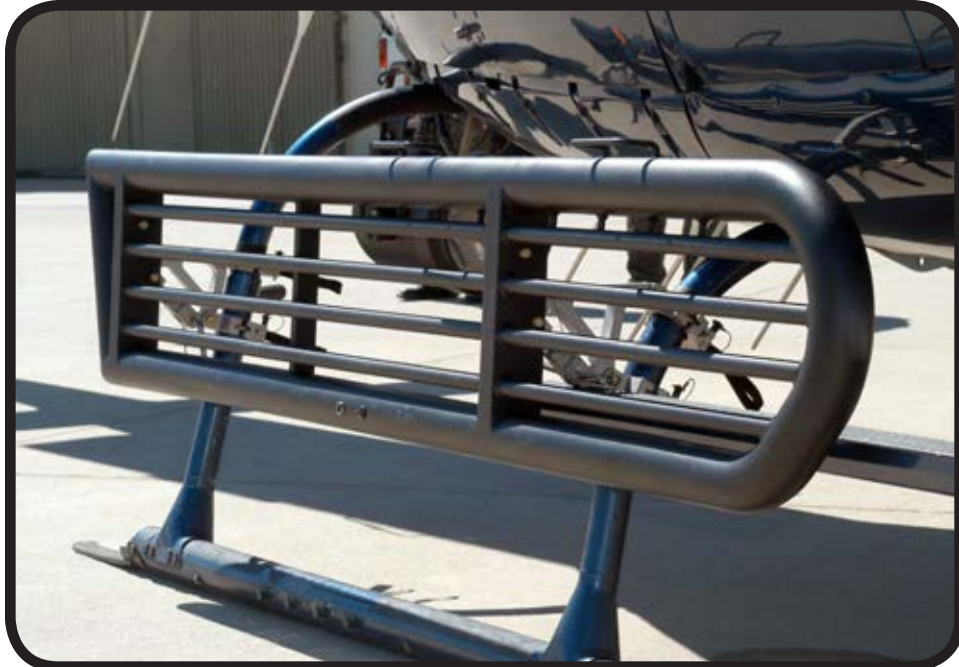
Cargo rack securely folded into stow position.
