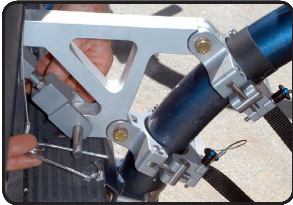
Insert lock-rod and secure with safety-clip. (repeat for assembly at other end of cargo rack)
