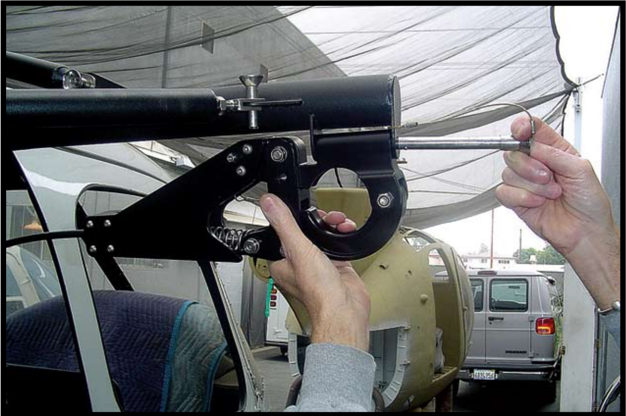
Large PIP pin holds hook assembly onto arm
