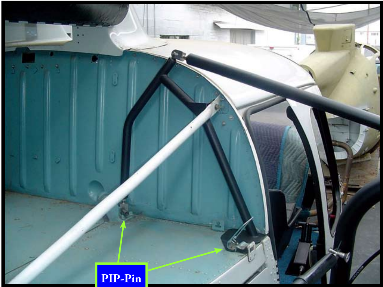
View of transmission compartment wth top “Y” brace installed. RIGHT SIDE SHOWN
