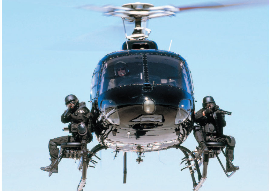
Law enforcement aviation units are increasingly adding an armed response capability. Two armed officers are seen here during a test of the innovative Tyler special operations platform.
