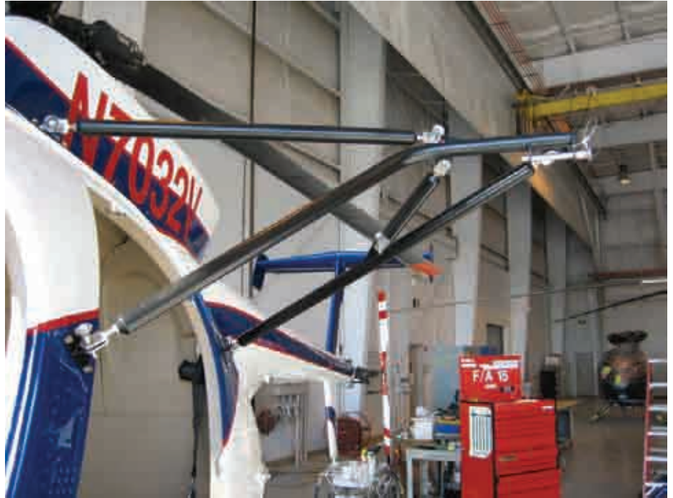
Figure 2. Left Side Installation of Frame
