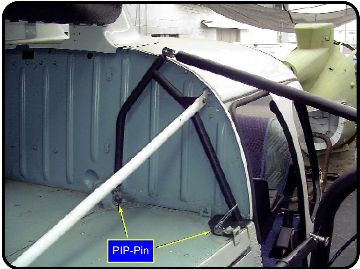
View of transmission compartment with TOP "Y" BRACE installed
