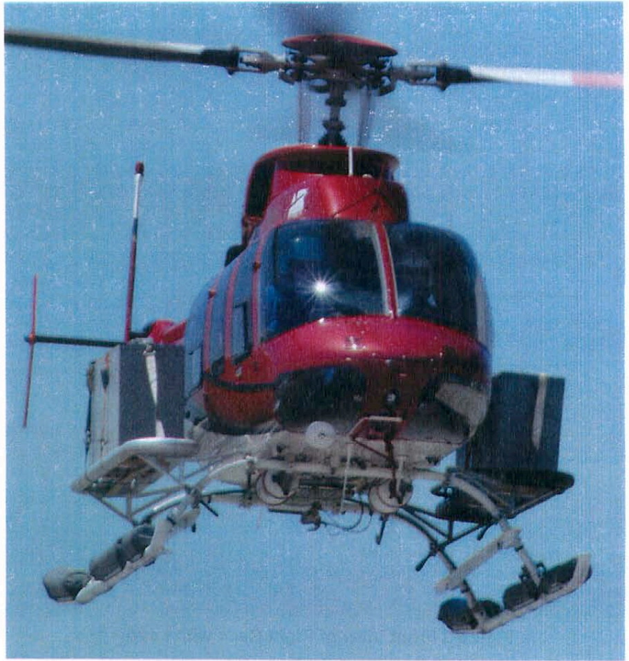
Figure 2 Front View of Installed Racks with Load
