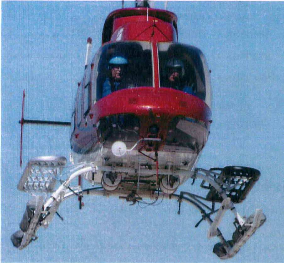
Figure 1 Front View of Installed Racks
